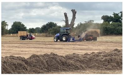
The morning was hot and dry and the contractors faced dessert like conditions. The 'field top maker', the machine which planes off all existing organic matter, created a veritable dust storm into which for a while the collecting vehicles completely disappeared.
